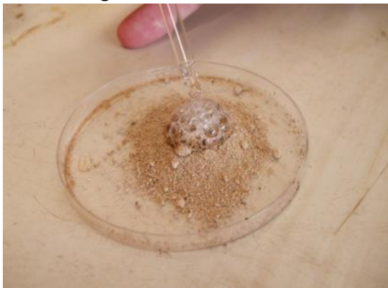
Figure 7. “Fizz” test for carbonates. .
