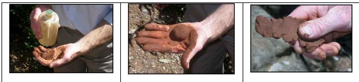
Figure 3. Hand texturing soil samples in the field
